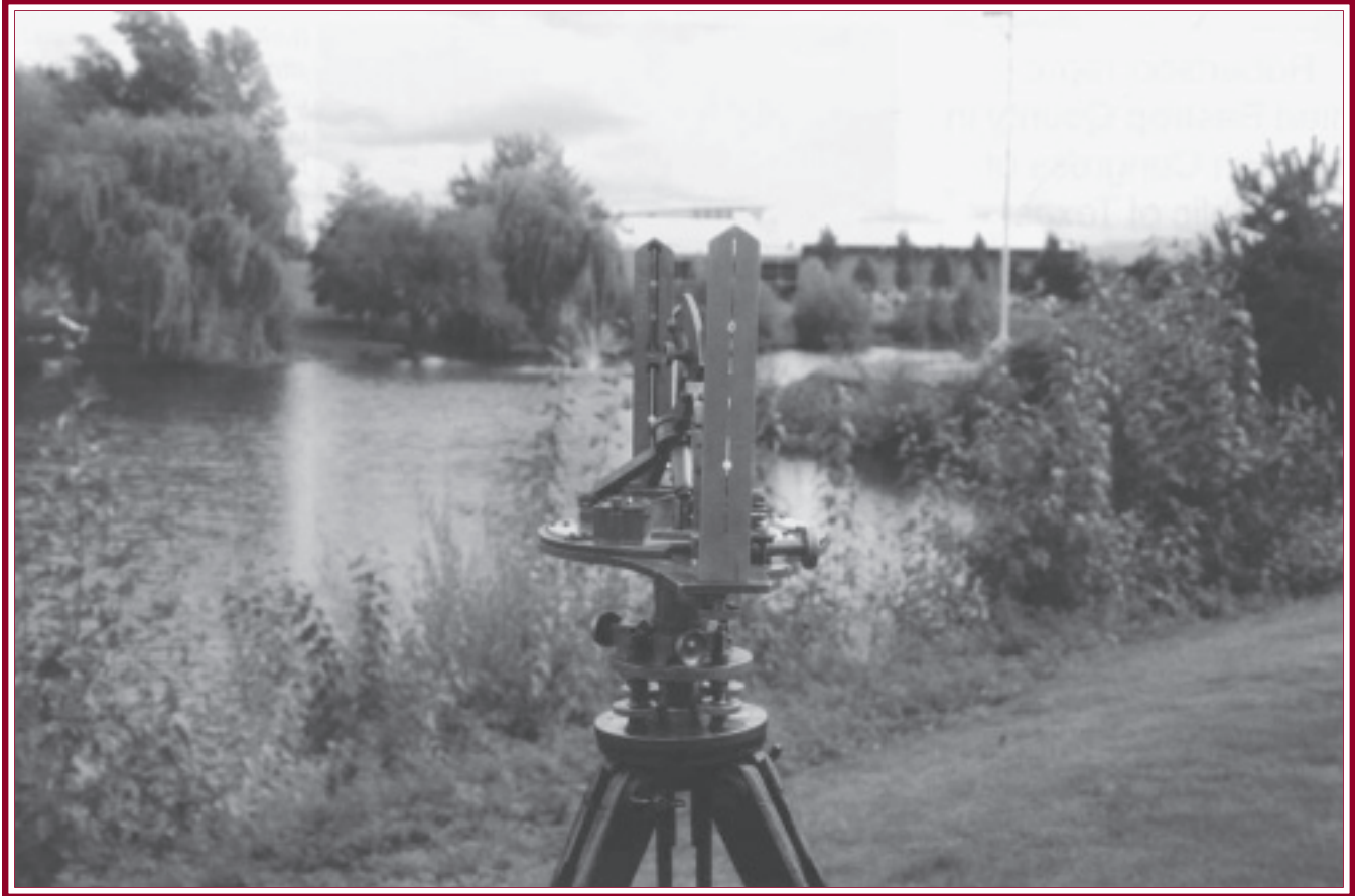
This is an operator's view of a solar compass. (Photos courtesy of Johnny Ingram)
