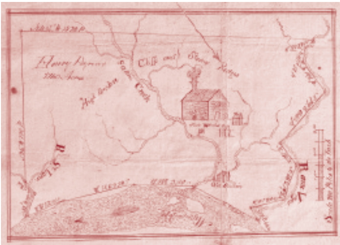
A plat of survey of an 1806 French Concession comprising some 1160 acres, located in the “Louisiana Territory, District of Ste. Genevieve”. In addition to the usual boundary measurement information, this plat of survey includes artistic depictions of existing commercial improvements, and locations of valuable water resources and ground features.
