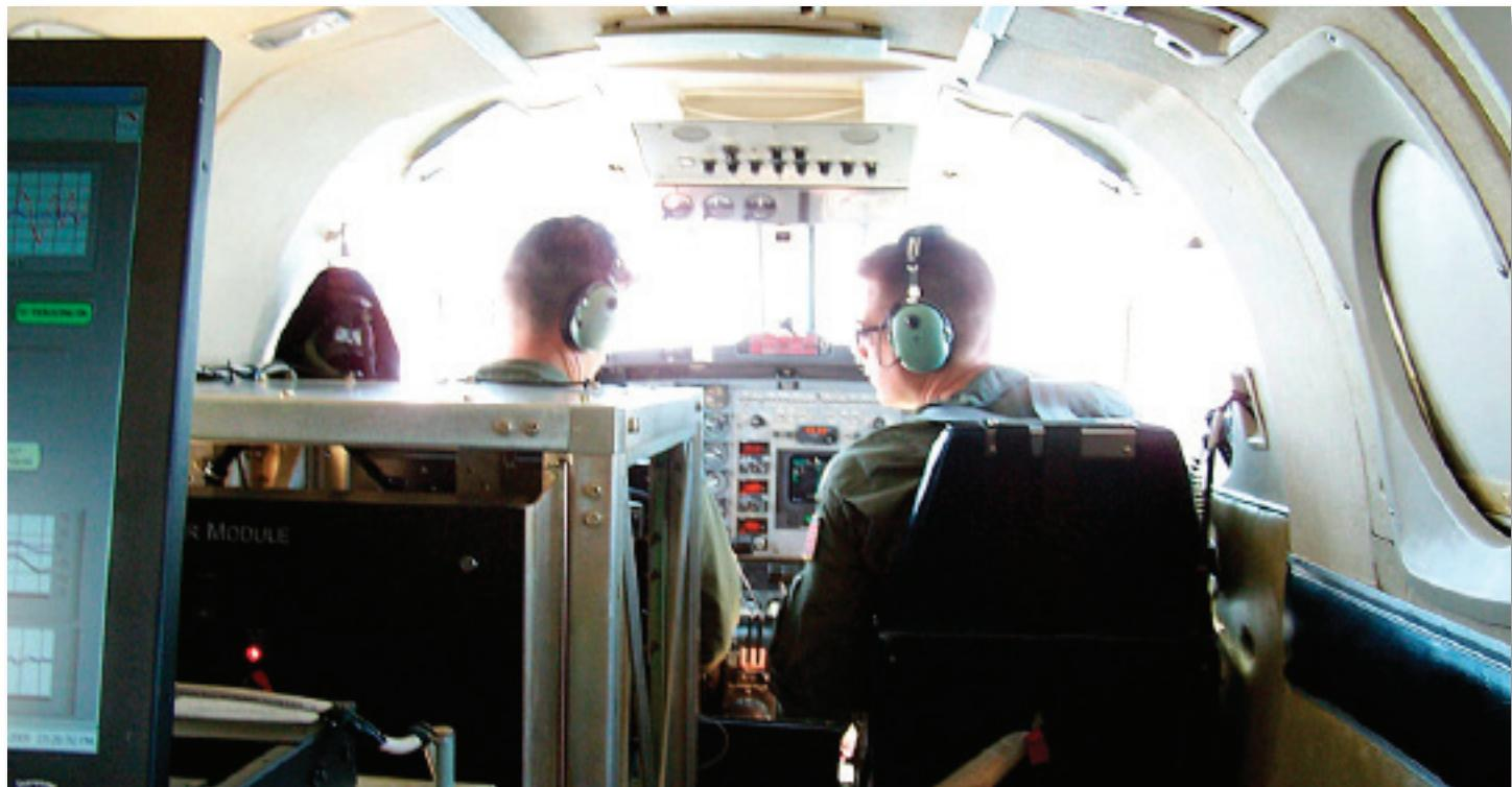
The pilot and co-pilot of a Navy-owned King Air aircraft prepare for takeoff on a data collection flight with GRAV-D instruments (fore and mid-ground) and a GRAV-D operator as their payload.
