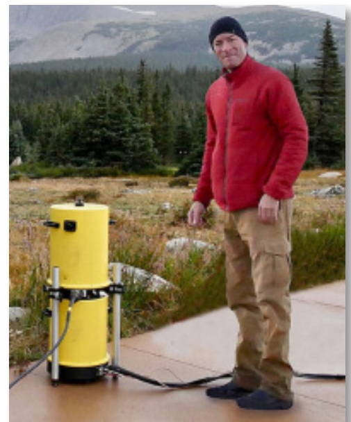
NGS geodesist and physicist Dr. Derek van Westrum calibrating a gravity meter in the high altitudes west of Boulder, Colorado.
